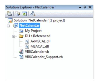
Before compiling the solution, check the "Instructions" region at the top of each class. In most cases, the project that AxWrapperGen utility creates compiles correctly at the first attempt. The compilation process creates a DLL that you must manually copy into the VB Migration Partner's main directory.
